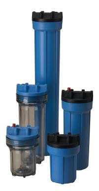
Pentair Slim Line<sup>§</sup> Filter Housings are available in either reinforced polypropylene or clear Styrene-Acrylonitrile (SAN) in 5", 10" and 20" lengths. The black or blue reinforced polypropylene housing caps are available with 1/4", 3/8" or 1/2" NPT connections. Four bosses are molded into every cap for mounting purposes.
